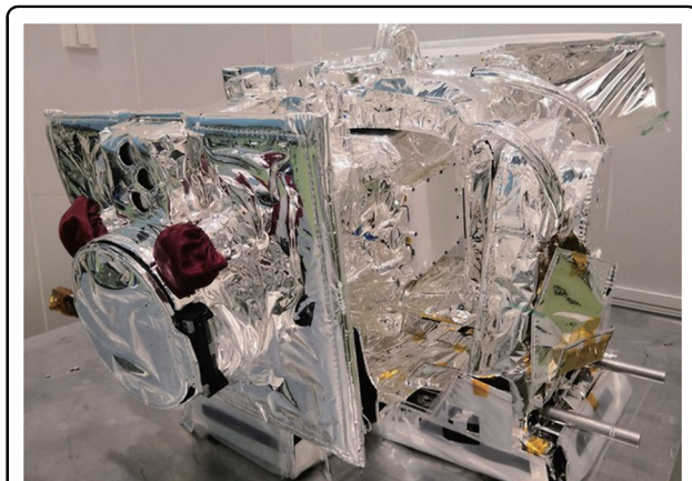
Fig. 2 The X-EUVI loaded onto the Fengyun-3E Satellite
